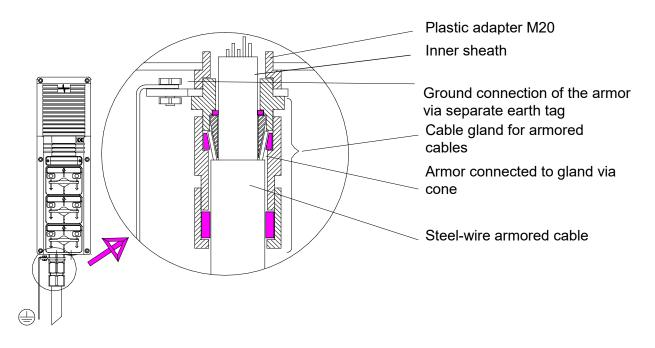
Metal cable glands which are installed in plastic housings (e.g. speakers or INDUSTRONIC intercom stations of the DAX series) must be grounded with additional grounding rings which are placed between the gable gland and the housing or by means of special cable glands with external ground connection.
