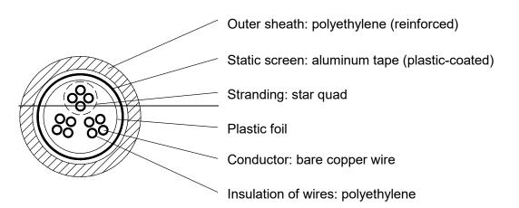
Please note: In case of star quad stranding, two opposite conductors form a pair (not the adjacent conductors).
